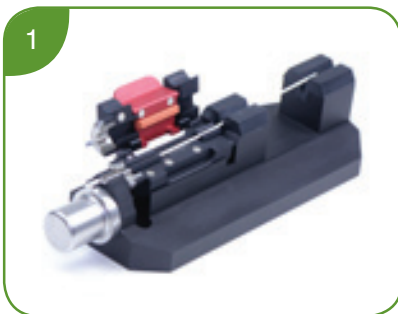
Place fiber into V-groove
